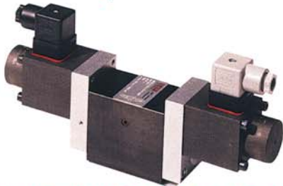
Bieri - Directional Seated Valve, 4/2 or 4/3 Positive Overlap, 100 % duty cycle Solenoid / Manually Operated NG 6, upto 700 Bar, upto 25 lpm
