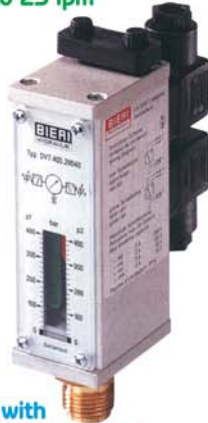
Bieri - Directional Seated Valve, 4/2 or 4/3 Positive Overlap, 100 % duty cycle Solenoid / Manually Operated NG 6, upto 700 Bar, upto 25 lpm
